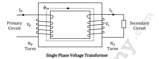
In other words, for a transformer there is no direct electrical connection between the two coil windings, thereby giving it the name also of an Isolation Transformer. Generally, the primary winding of a transformer is connected to the input voltage supply and converts or transforms the electrical power into a magnetic field. While the job of the secondary winding is to convert this alternating magnetic field into electrical power producing the required output voltage as shown.
